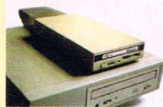
The CDPlus and SyQuest EZ135 drives. The IDE Zip Drive is the same size as the EZ135
